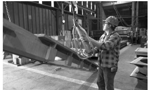
Positioning large cast frame for machining
